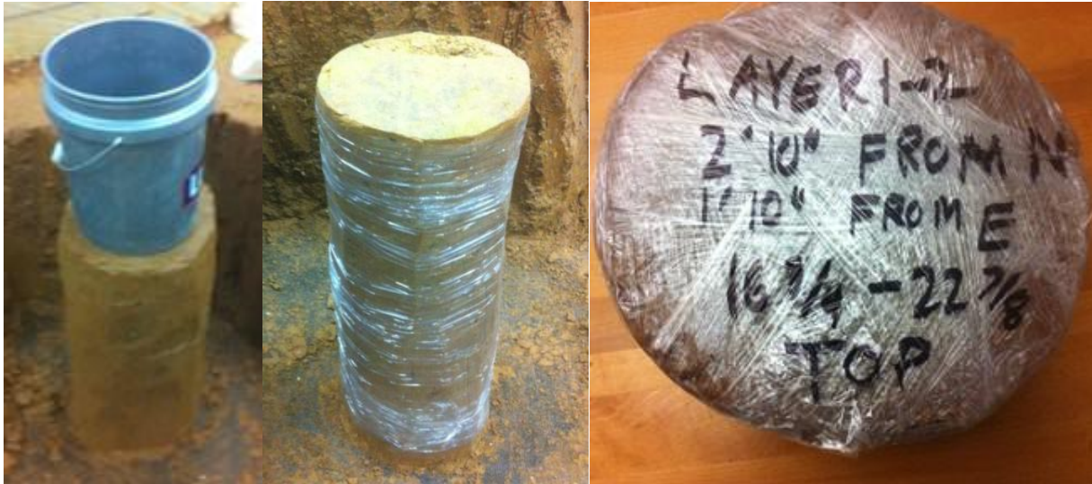
(a) (b) (c) Figure 3.33. (a) Rough column with bucket for a guide, (b) hand carved soil column wrapped in plastic wrap, and (c) soil block wrapped in plastic.
