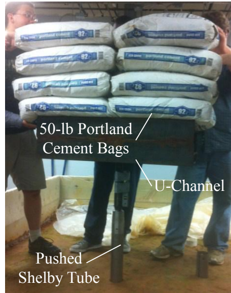
Figure 3.31. Shelby tube pushed into Test Pad 2.
