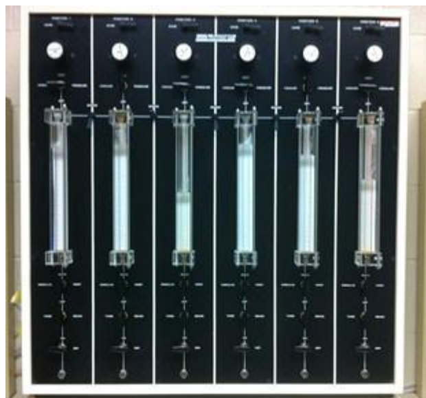
Figure 3.4. Trautwein panel boards used for laboratory hydraulic conductivity testing.
