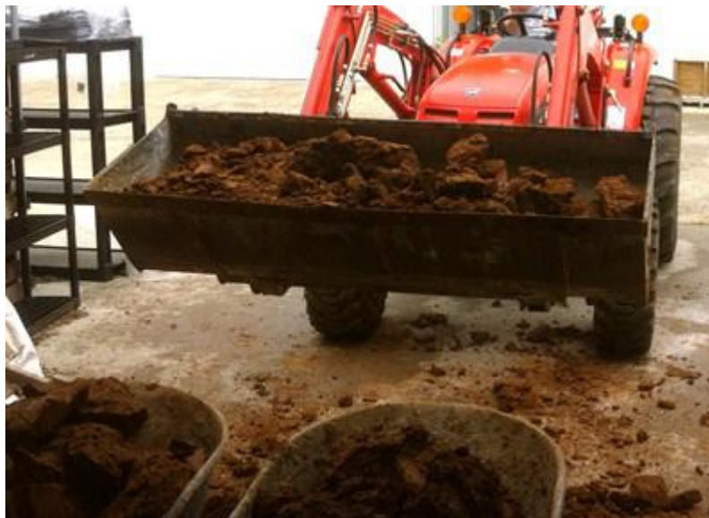
Figure 3.15. Soil being transferred from wheelbarrows to the front bucket of the tractor.
