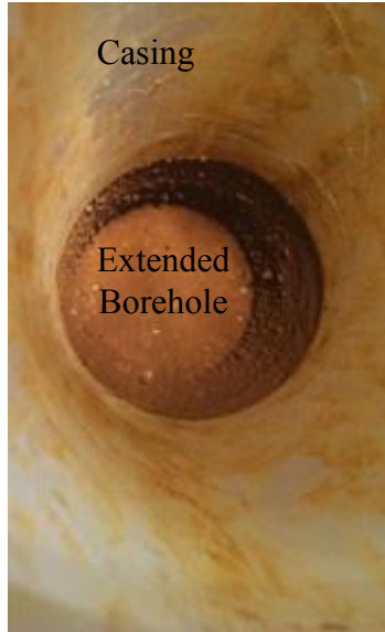
Figure 3.19. Photo of extended borehole.
