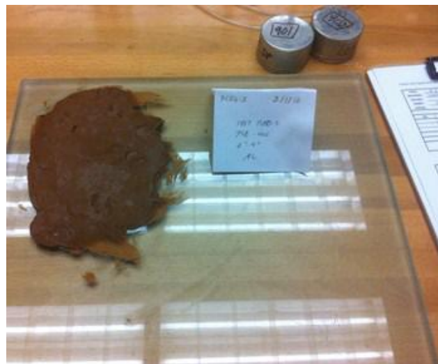
Figure 3.45. Soil sample drying for plastic limit testing.
